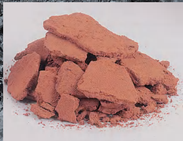
脱水后的泥饼 Sludge cake after dewatering
