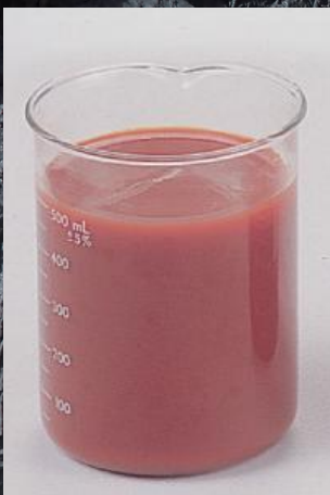
脱水前的污泥水 Sludge water before dewatering
